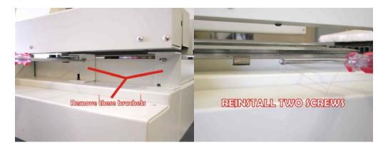
3. Install the sheet trays onto the top of the main machine tube you will need to use the screws already installed into the tube
